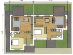
Floor Plan-Proposed Type 1 (scale 1:200)
