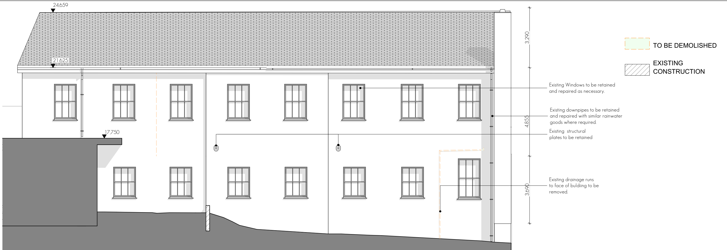
Existing-Demolition South (Rear) Elevation
