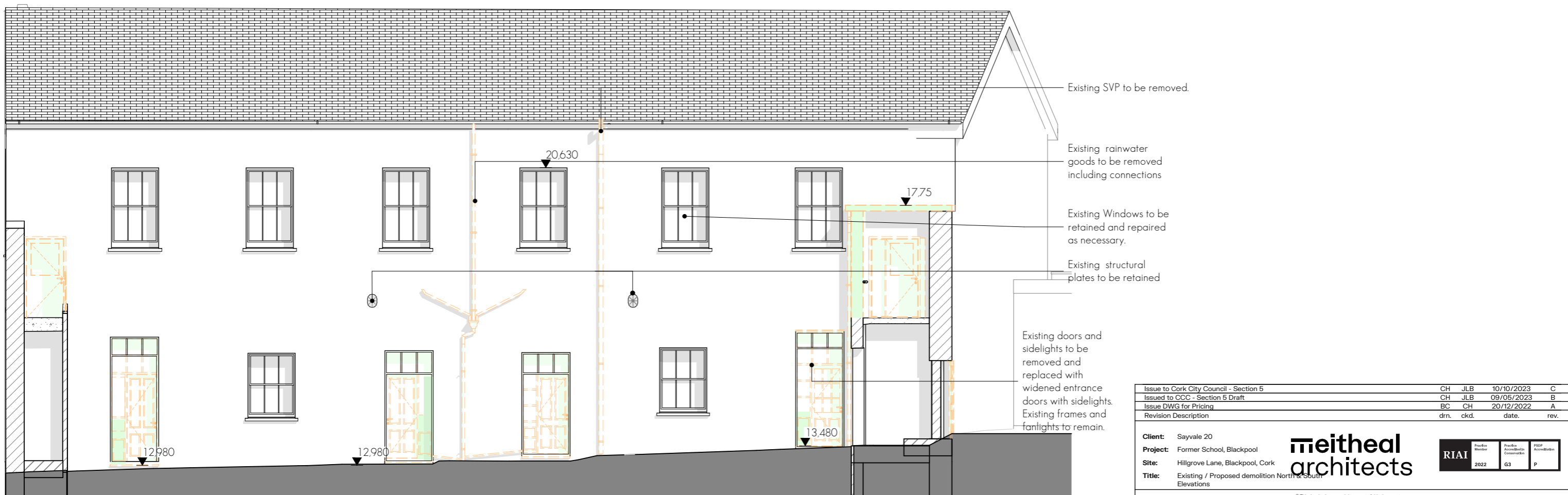
Existing-Demolition North (Front) Elevation
