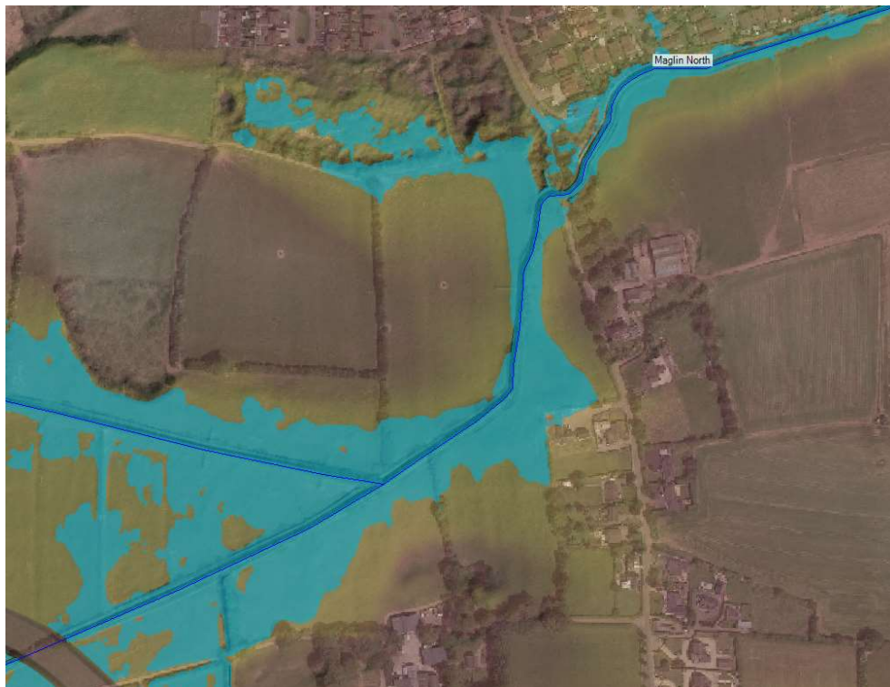
Figure 11.8: 1% AEP MRFS Flood Extents – Maglin Road Bridge Blockage
