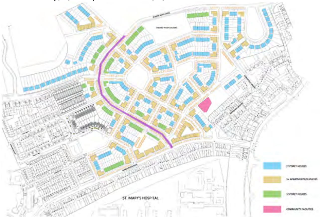
Fig.3 CNWQR Masterplan, distribution of residential units; route of proposed 'Spine' road shown in purple
