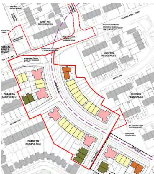
Fig. 7 proposed Phase 1C site layout, with interim Kilmore Rd intersection at the top
