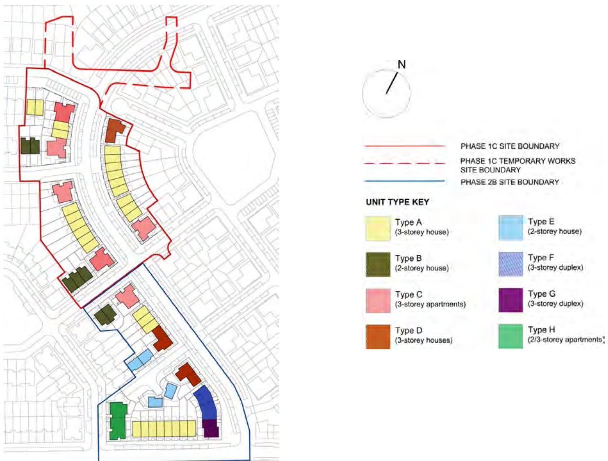
Fig.6 Key plan showing unit type within Masterplan context; Phase 1C is outlined in red, phase 2B in blue
