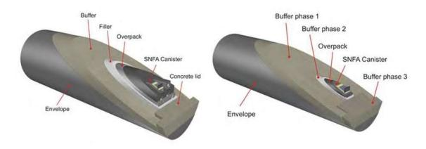
Figure 30: Supercontainers for spent fuel if considered waste: a supercontainer can hold 4 UOX fuel bundles (left) or 1 MOX fuel bundle (right)<sup>lix</sup>.
