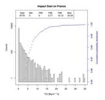
Figure 22: Distribution of the maximum time-integrated concentration (TIC) in France after a hypothetical 6-hour discharge of radioactive noble gases from the Doel nuclear power plant. The total number of TIC values shown in the distribution is 8,<sup>77930</sup>.
