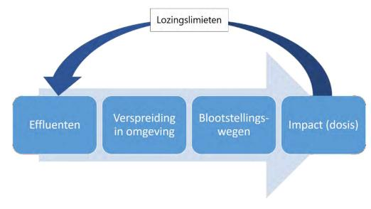
Figure 14: Steps in methodology for radiological impact of discharges in normal operation.
