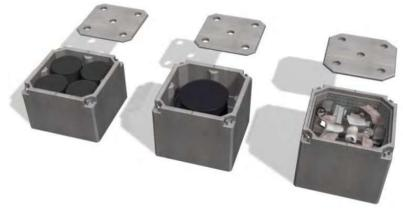
Figure 27: Illustrations of the three types of <sup>caissonsivi</sup> containing waste: type I (left), type II (center) and type III (right). After placing the lid and filling the space between waste and caisson with filler mortar, these disposal colli are called "monoliths."
