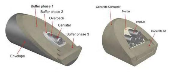
Figure 29: Supercontainer for vitrified waste (li nks)<sup>lix</sup> and monolith-B for compacted waste (right)<sup>lx</sup>.
