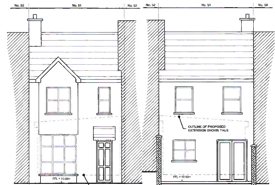
EXISTING DWELLING HOUSE - FRONT ELEVATION SCALE 1:75
