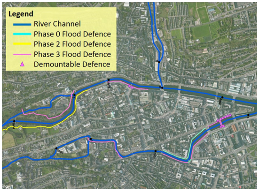
Figure 32: Defence lines and demountables – Phase 3
