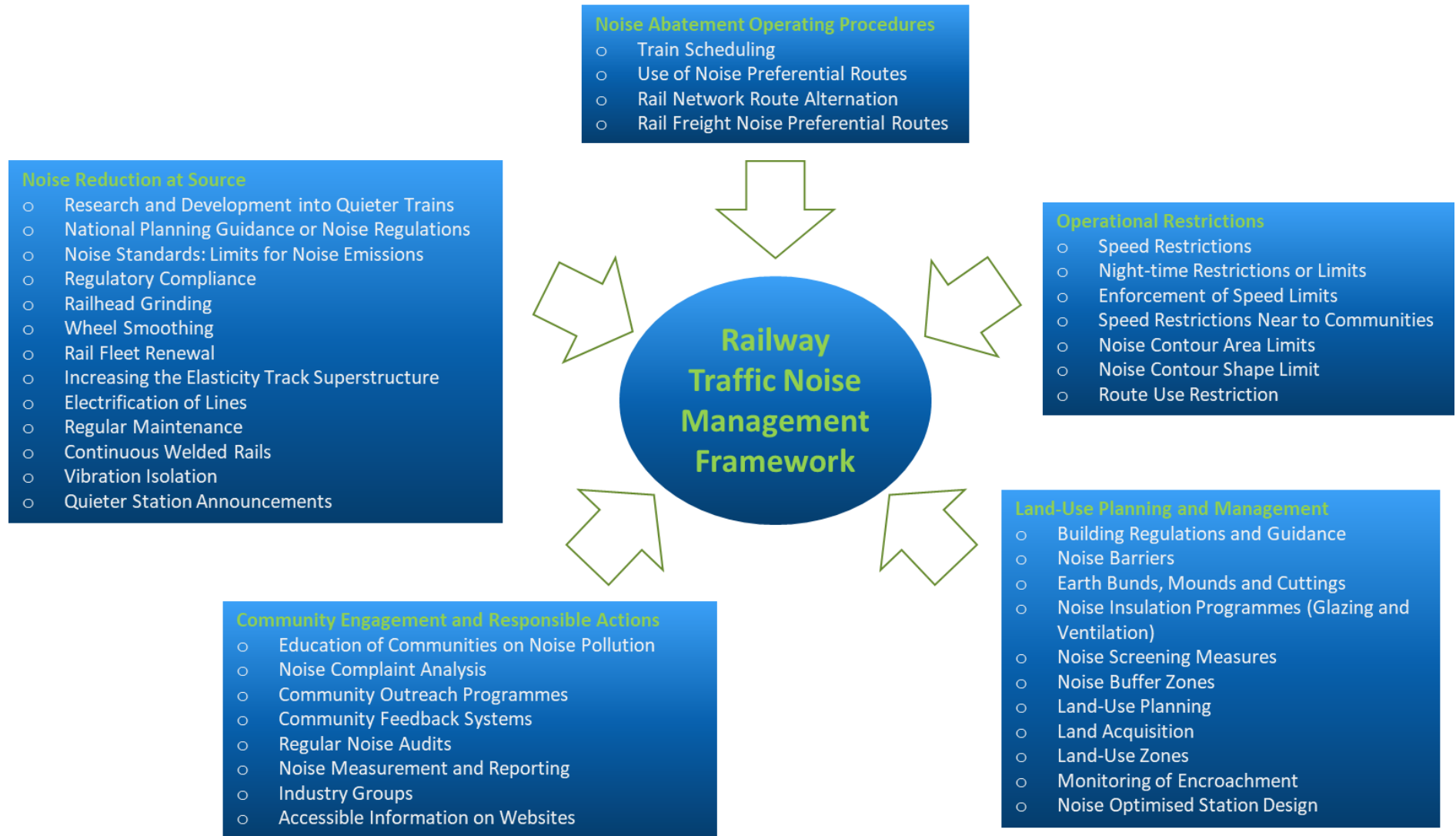
Figure 14: Railway Traffic Noise Management Framework
