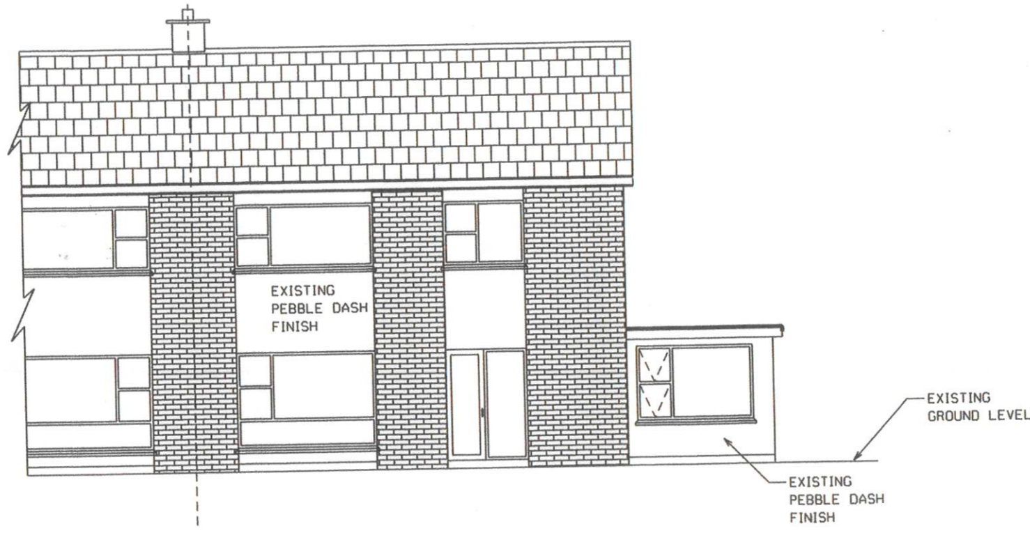
EXISTING NORTH ELEVATION
