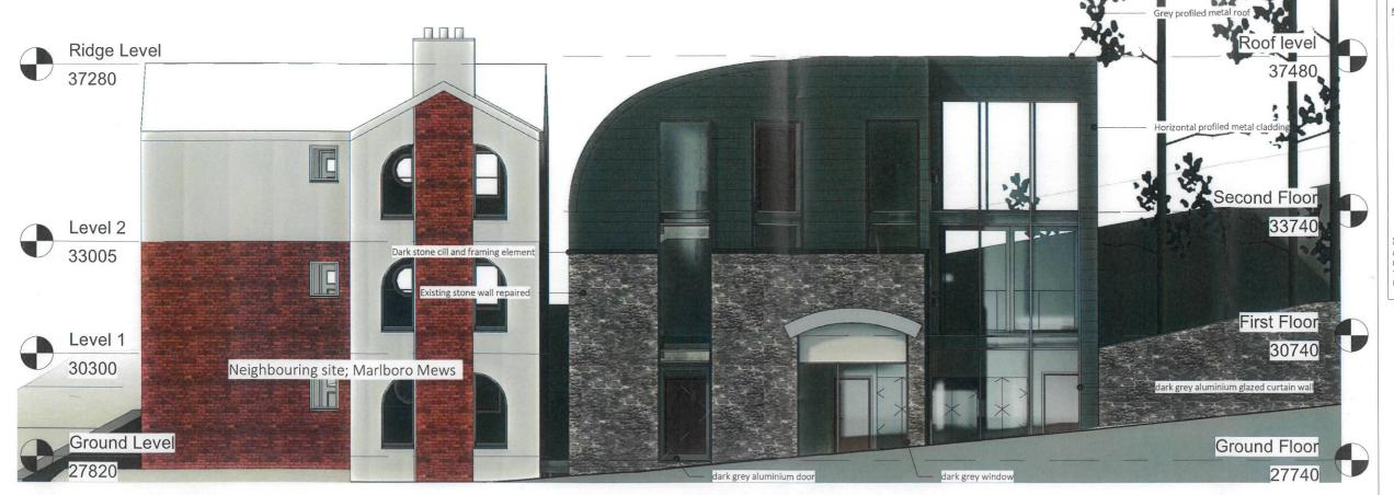
Proposed Front Elevation Roof level Grey profiled metal roof Ridge Level 37280 Second Floor 33740 Level 2 33005 First Floor Level 1 30740 30300 Neighbouring site; Marlboro Mews Ground Level Ground Floor 27820
